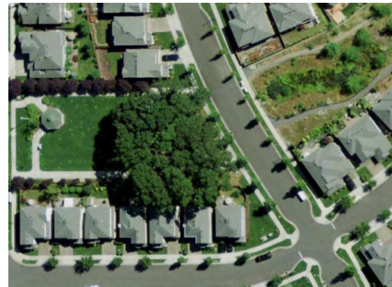
In this example, the careful arrangement of site features (streets; laneways; open space; walkways; residential lots; park; and, trails), creates improved street end views, attractive streetscapes, and connections between uses. The uses are not arranged to be segregated, but interconnected. Source: Google
