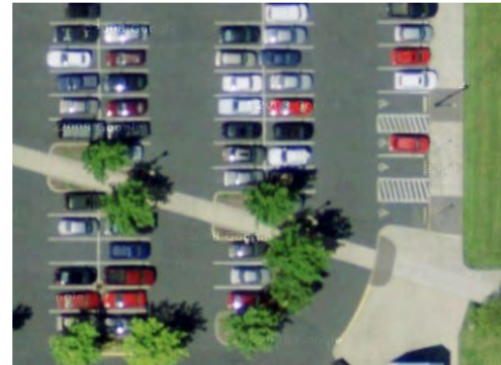
The diagonal walkway in this photo provides a link between a main pedestrian route to a building entrance, while also providing a safe walking environment through the parking area. Source: Google
