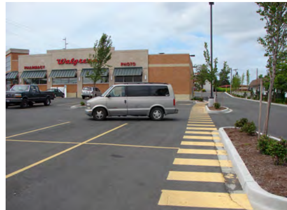
Use of pavement markings and shy distance around planters to create a safe travel route for pedestrians in a parking lot.
