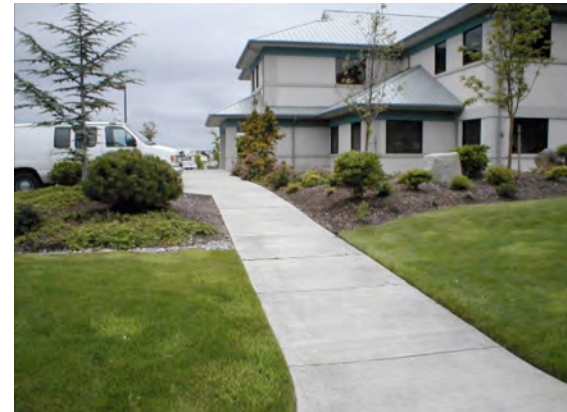
Example of an entrance that does not require pedestrians to cross through a parking area to gain access from the sidewalk.
