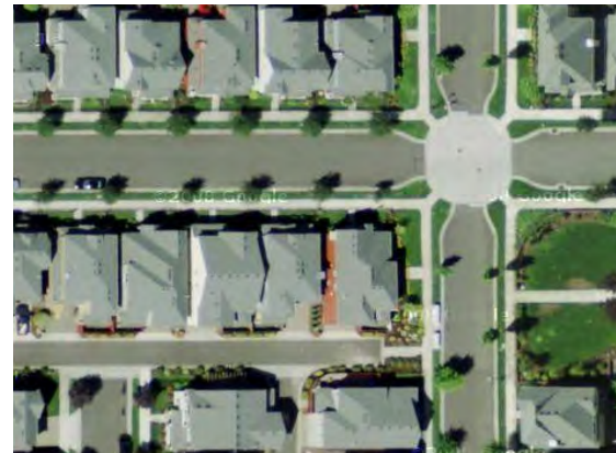
Pedestrian access and safety is improved in this location with: a. the use of curb extensions to reduce crossing distances and traffic speeds; b. sidewalks; and, c. a pedestrian scramble at the main park entrance. Source: Google
